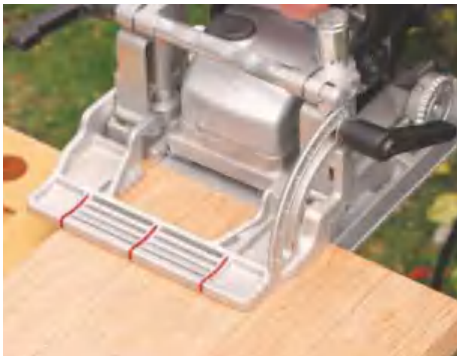
STEP 7. Cut slots for biscuits in the ends of the rear panel. These are for attaching the end pieces later
